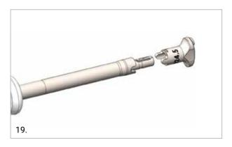
Slide the M5 Fixation Rod into the assembled Baseplate impactor.
