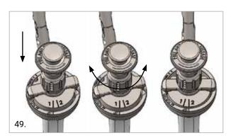
In case it is difficult to remove the stem from its slot, insert the Backtable Assembly Block in the Backtable Stem Removal Device and screw both components. This will push the stem up and release it from the block.
