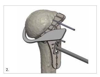
Perform the cut using an oscillating saw.
