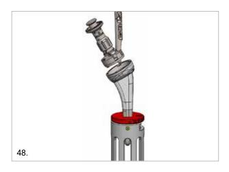
Push the handle down towards the implant and, holding it down, rotate the instrument clockwise aligning the "2" line to the medial line of the implant. The instrument is correctly connected when a snap is felt.
